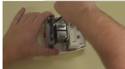
Fit the supplied batteries (2 x "C" cells). Note, the correct orientation is marked in the battery compartment. The motor will turn for around five seconds.
