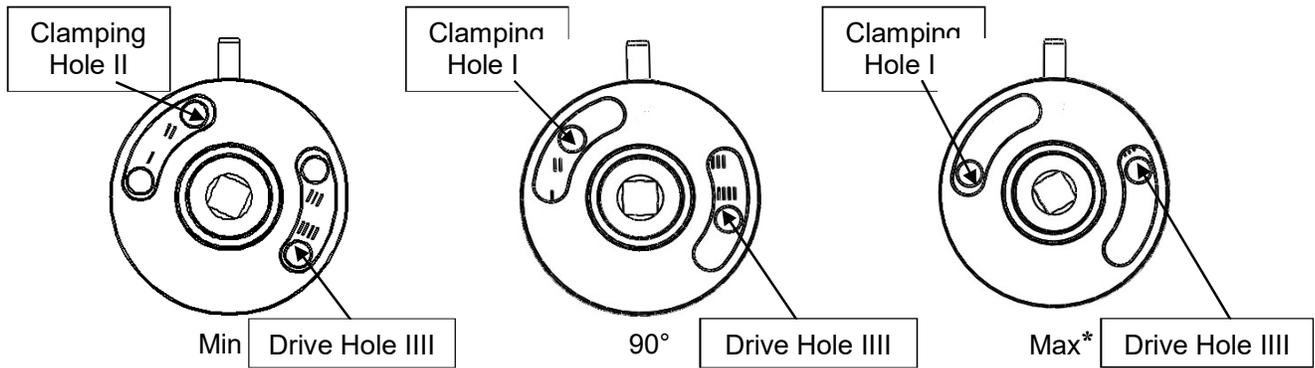
Figure 4: Right Hand Parallel Arm Cam Positions
