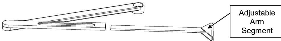
For parallel arm configuration, fit the parallel bracket to the door frame using the 3 x N°10 \* 1" wood screws and then fit the adjustable arm segment to the bracket using the 2 x M5 \* 6 foot screws
