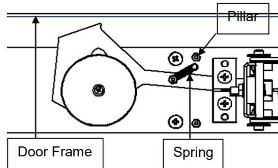
Separate the door closer arm and fit the adjustable arm segment to the door frame using 2 x N°8 \* 1-1/4" screws.
