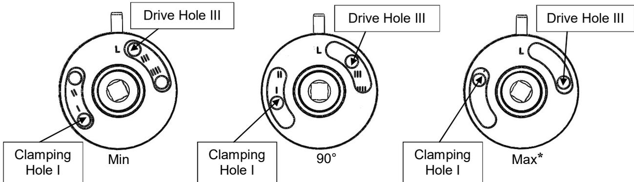
Figure 1: Left Hand Projecting Arm Cam Positions
