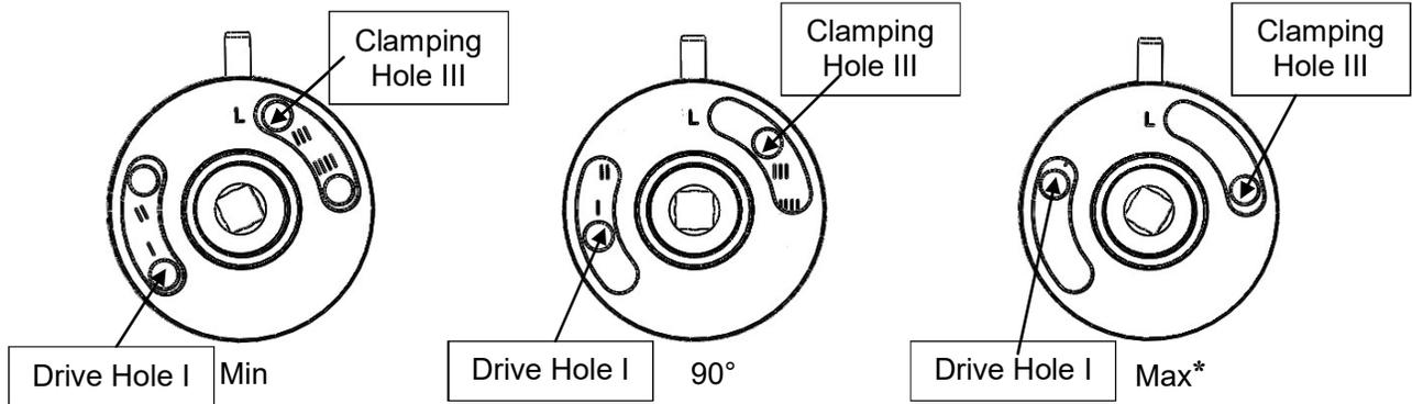
Figure 3: Left Hand Parallel Arm Cam Positions
